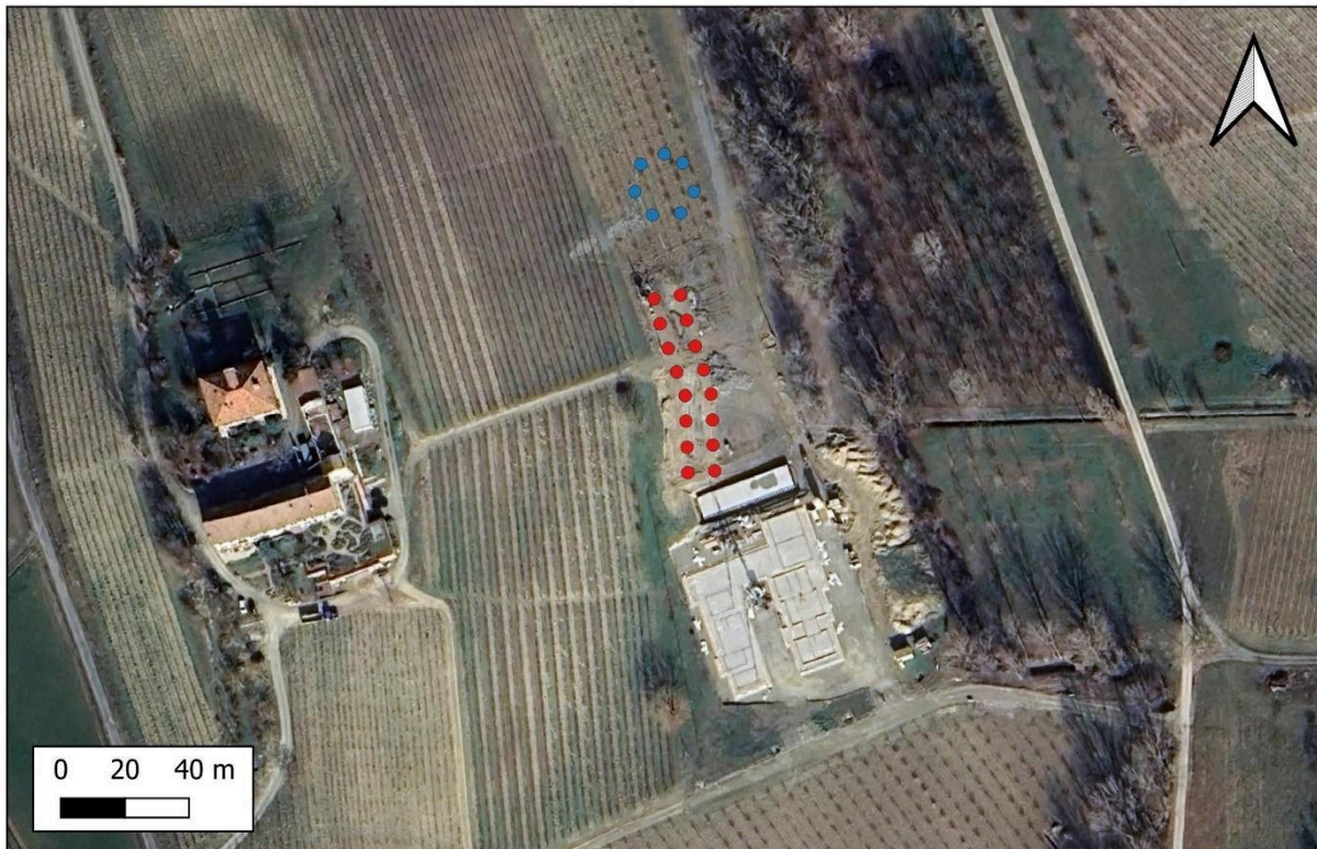
Figure 2.9 – Satellite image of the new development area with location of the 16 BHEs of the conventional GSHP system (red dots) and the 7 BHEs of the experimental BTES (blue dots).
